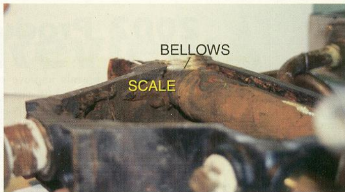
Bisected McDonnell Miller low water cut-off switch. Note scale formation.
